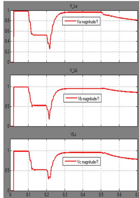
Figure 13.2. Load Voltages of phases during open circuit fault with Controller
