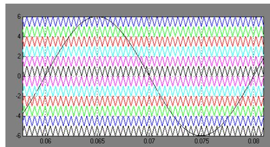
Figure 3. Reference waveforms for 13-level cascaded H-bridge converter
