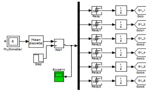
Figure 8. Controller to generate signal for the bypass switches
