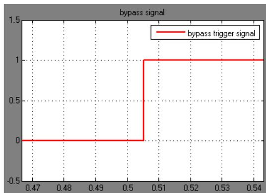
Figure 15. Relay operation signal during open circuit fault at 0.5sec
