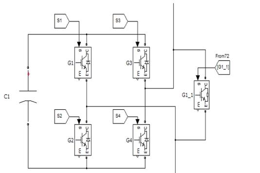
Figure 7. H-bridge with bypass IGBT switch
