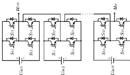
Figure 2. Multi level cascaded H-bridge converter of one phase
