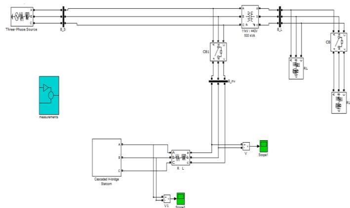
Figure 9. Simulink modeling of test system
