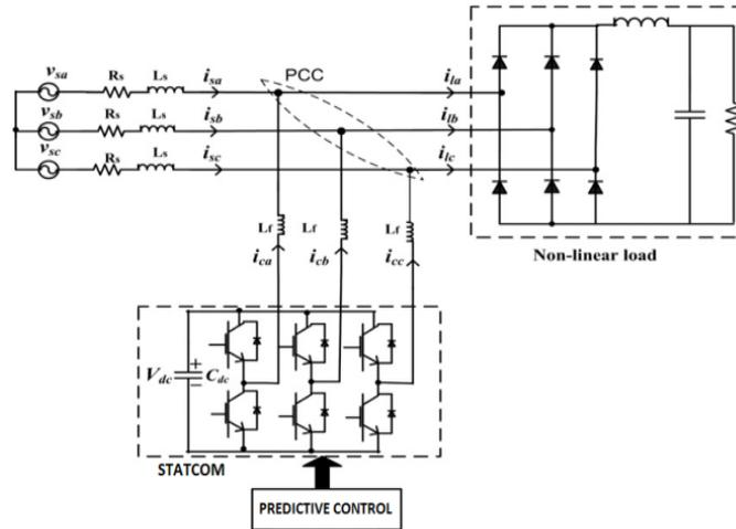
Figure 1. Block diagram of test system
